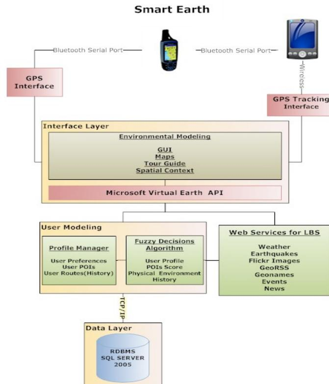
Fig. 1. Functional Schema of the Smart Earth
